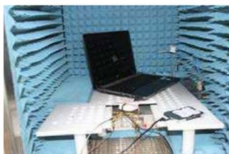
Figure 7: The measurement setup for the noise power.
