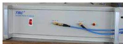
Figure 8: The auxiliary device of the microwave power clamp, SNA.
