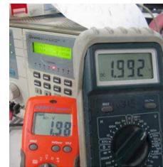
Figure 9: balance voltages across completely charged super-capacitors.
