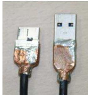
Figure 17: The improved termination scheme for mitigating USB 3.0 EMI problem.
