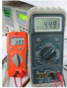
Figure 4: Voltages across completely discharged super-capacitors.
