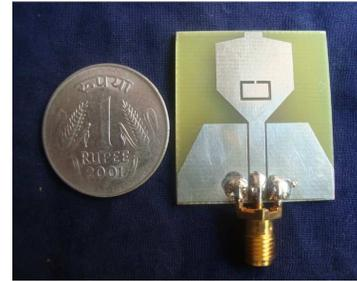
Figure 2: Photo of fabricated antenna.
