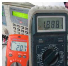
Figure 8: Imbalance voltages across completely charged super-capacitors.
