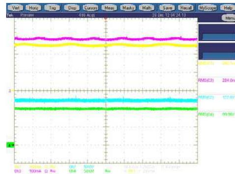
Figure 6: Current and voltage waveforms for two LED strings.
