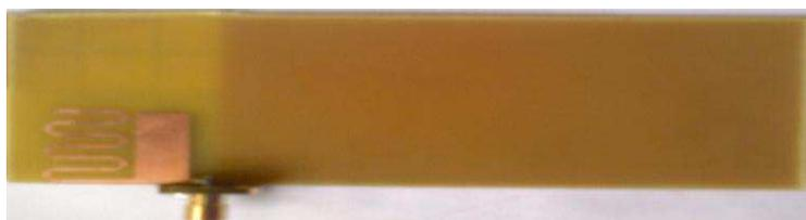
Figure 2: Photo of the fabricated antenna.
