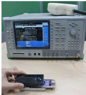
Figure 11: The test setup of display module near field EMS.
