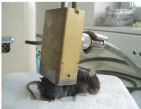
Figure 1: Waveguide applicator for biological experiments.
