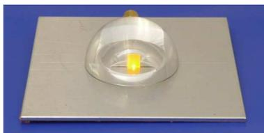
Figure 2: A photo of the DRA prototype. An LED is inserted into the hollow region of the DRA to serve as the light source.
