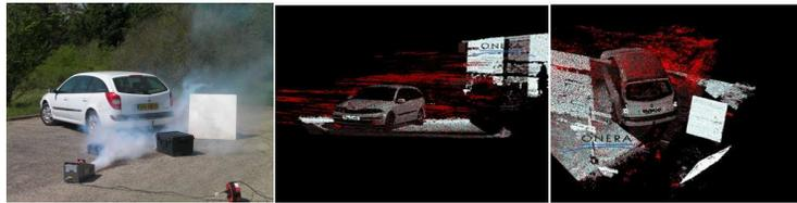
Figure 7: Detection of a vehicle and identification of the fog contribution (red dots).
