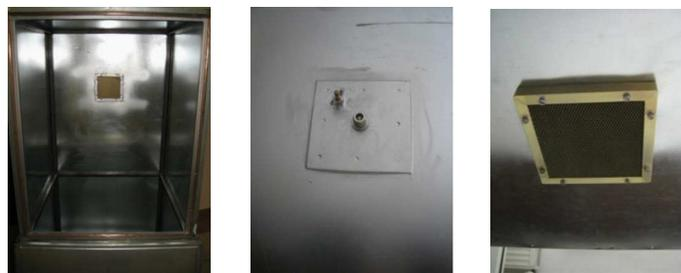
Figure 2: View of the interior of a small shielding chamber with a transit panel and Honeycomb filter.
