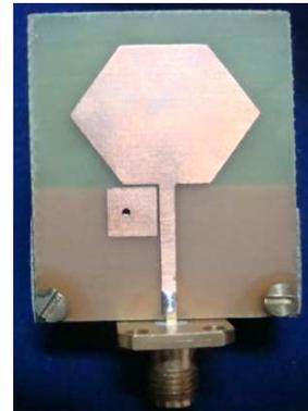
Figure 2: Photo of fabricated antenna.
