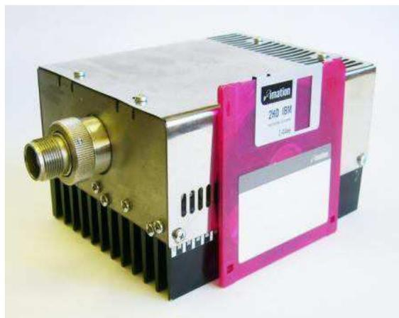
Figure 3. Gin10-50-100 [2] generated pulsed of about 10 kV (with rise time of 50–70 ps) with repetition pulses up to 100 kHz. Output feeder is HN-connector.
