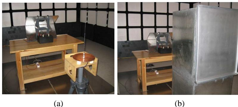
Figure 5: The laboratory stand for the measurement of shielding effectiveness of small shielding chamber in the anechoic chamber: (a) standardization measurement, (b) proper measurement.
