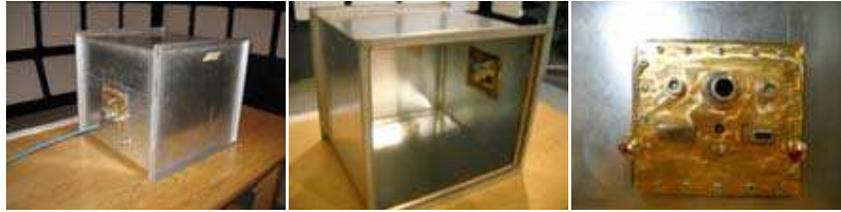
Figure 8: View of the studied shielded chamber with terminal panel.
