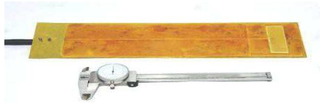
Figure 4. Linear strip transducer of LTF2 for measurement of the  $\mathbf{E}(t)$  pulse electric field in TEM traveling wave. Sensor parameters:  $\mathbf{T}_f \approx 20$  ps — transient response rise time;  $\mathbf{T}_{\max} = 2.8$  ns — time of measured interval;  $\mathbf{K}_{LTF2} = 0.4$  V/(kV/m) — sensitivity; 0.5 m — outer cable length to connect.
