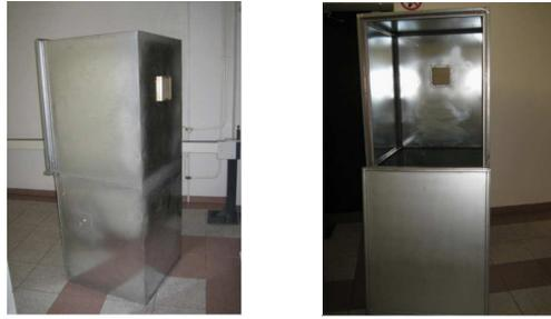
Figure 1: Small chamber shield used as a model of the case RACK-type.
