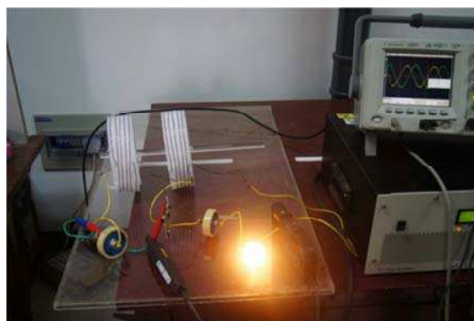
Figure 5: The experiment figure, the current phase of transmitting coil is ahead of receiving coil \pi/2 .
