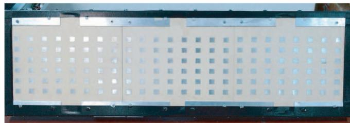
Figure 2: Front view of UAVSAR antenna with supporting structure.
