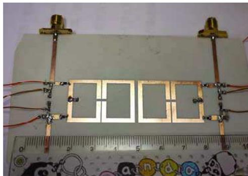
Figure 2: Photograph of the DPDT filter-integrated switch A.
