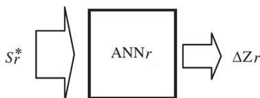
Figure 3:  $ANN_r$  as a mapper of detuned scattering characteristics to tuning element deviations that caused detuning.
