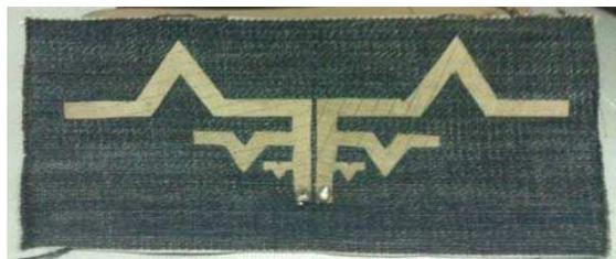
Figure 1: Multiband wearable antenna design.
