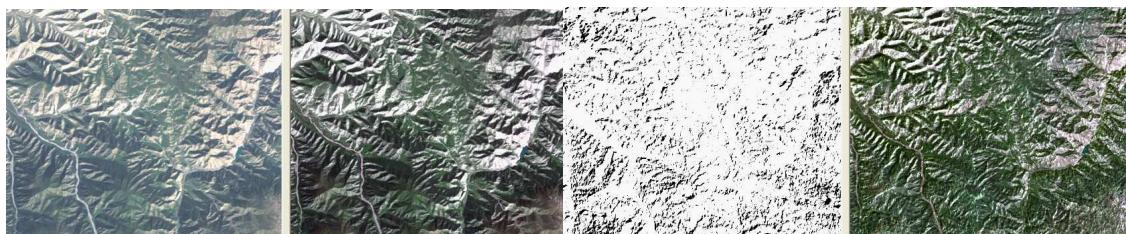
Figure 3: Original TM image, atmospheric correction image, BRDF correct factor and topographic correction image (from left to right).
