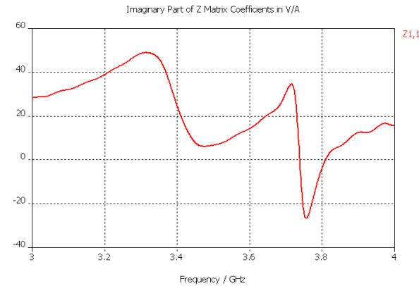
Figure 4: Imaginary part of the input impedance.
