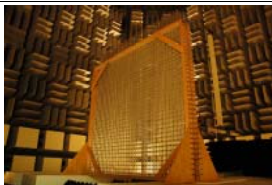
Fig.8 EM screen made of aluminum pipes with 1cm diameter and 2m lengths.
