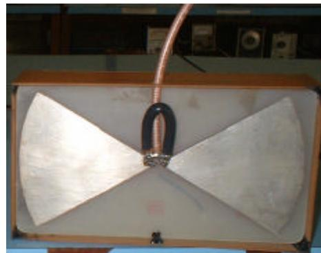
Figure 3. 1 – 2 GHz Circular end Bowtie Antenna
