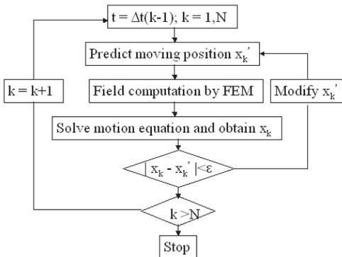
Figure 2: The flow chart of direct coupled method
