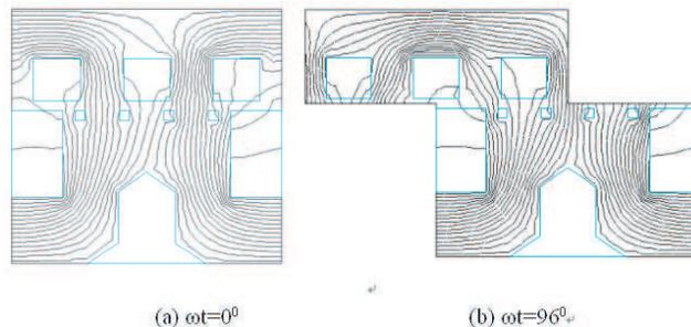
Figure 5: Flux at different time in electrical angle.
