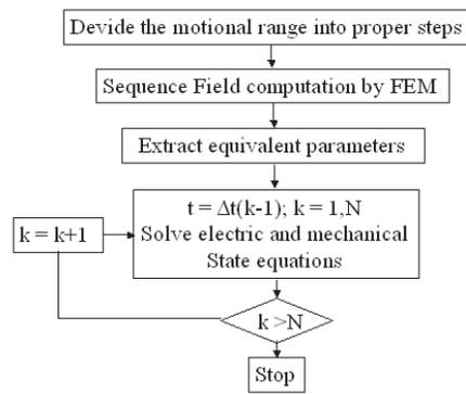
Figure 3: The flow chart of the fast solving technique
