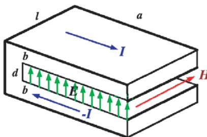
Figure 1: Horseshoe optical nanoantenna is excited by magnetic field  $\mathbf{H}$ ; arm length  $a$ , arm thickness  $b$ , lateral size  $l$ , gap width  $d$ ; electric current flows in metal arms; displacement currents in the gap short the circuit; magnetic moment of the current is either parallel ( $\mu > 0$ ) or antiparallel ( $\mu < 0$ ) to  $\mathbf{H}$ .
