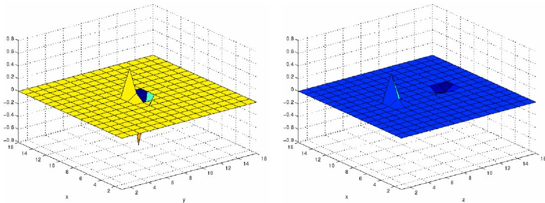
**Figure 2.** Wavelet coefficients of the projection  $Q_{m+1,z} P_{m+1,y} Q_{m+1,x}(-\rho)$  shown in the  $(x,y)$ -plane for  $z=6$  (left) and in the  $(x,z)$ -plane for  $y=8$  (right).
