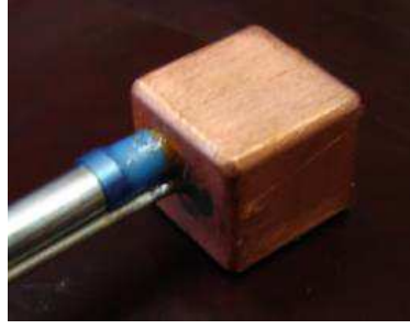
Figure 1: The measured Cu sample, 10 \times 10 \times 10 mm.
