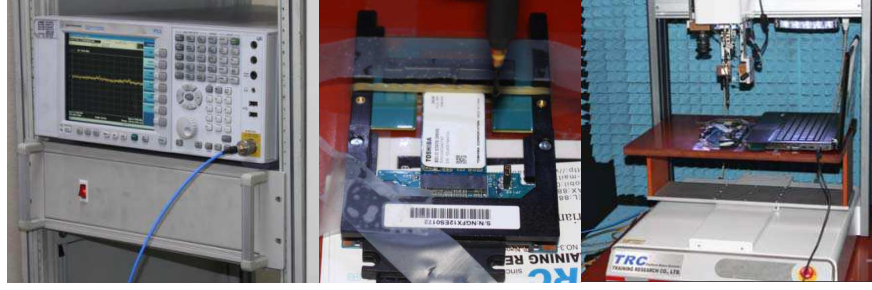
Figure 8: Circuitry and cavity resonance coupling measurement.
