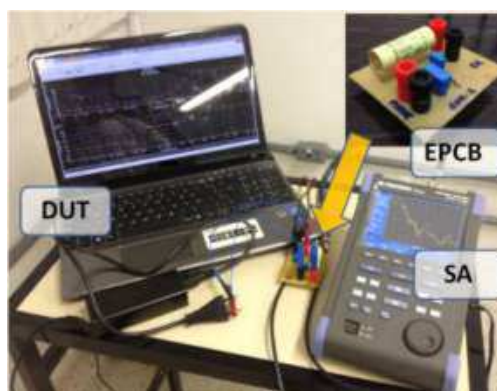
Figure 2: Conducted emission test setup using an EPCB.
