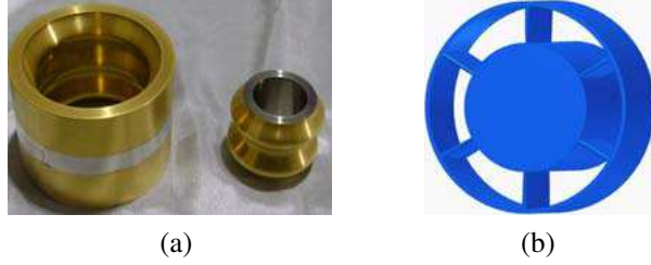
Figure 4: Important technical improvement in experiments. (a) Outer and inner ripples coated with the TiN film. (b) Close-up view of equipotential support in Figure 1.
