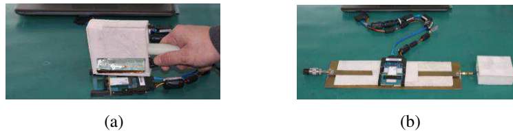
Figure 5: (a) Portable SG device for SSD EMS test. (b) Configuration of Stripline for SSD EMS test.
