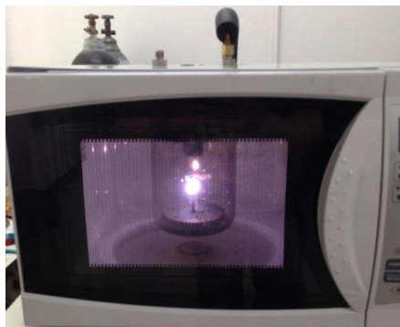
Figure 4: Photograph of plasma generation in ethanol vapor.
