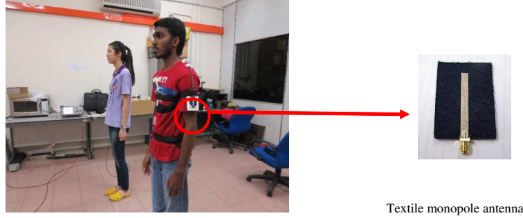
Figure 1: Measurement setup utilizing TM antennas worn on two subjects' bodies in indoor environment.
