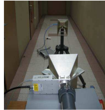
Figure 2: Block diagram of measuring position for wall attenuation in closed spaces in the configuration for basic measurement.
