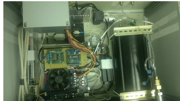
Figure 6: The picture of TDLAS detection system for early forest fire.
