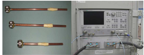
Figure 2: Handmade probes and network analyzer.
