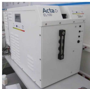
Figure 2: The hydrogen generator ACTA EL100c + dryer.
