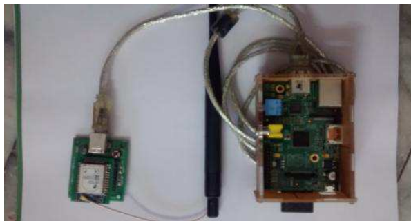
Figure 7: CDAU — Central Data Acquisition unit prototype and set-up.
