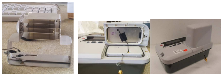
Figure 8: Left bare antenna supported by plastic clip of the left, centre antenna mounted in hood, right antenna housed in assembled gas meter.
