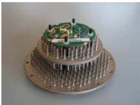
Figure 3: Dual band patch antenna with comb substrates.
