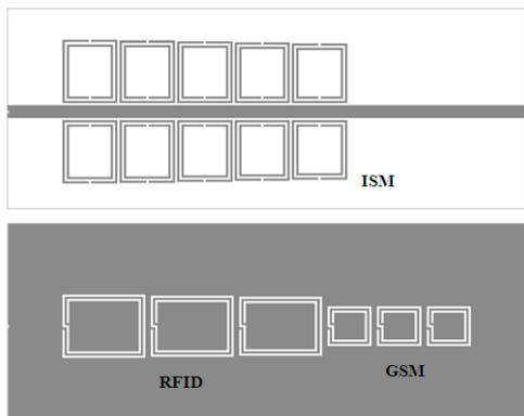
Figure 1: Topology of the designed multiband microstrip EMI filter. (a) Top layer with microstrip line and the SRRs designed at 2.45 GHz. (b) Bottom layer with CSRs etched in the ground metal tuned at 900 MHz and 1.8 GHz, respectively. Metallization zones are depicted in grey.
