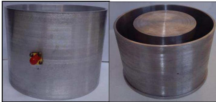
Figure 5: Fabricated input cavity.
