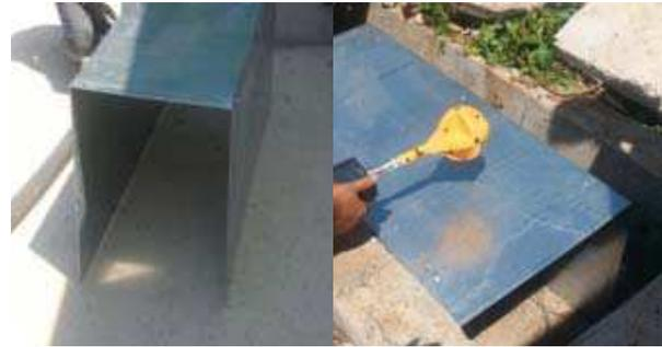
Figure 2: Measurement in the high voltage channel with reversed U galvanized shielding.
