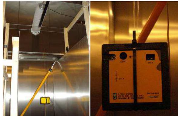
Figure 2: Method 2 — sensor fixed using plastic clamp and three fishing lines.
