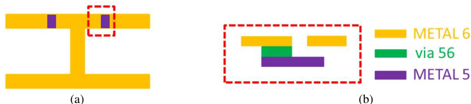
Figure 4: Schematic (a) top and (b) cross sectional views of unit cell.
