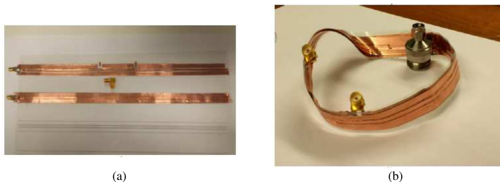
Figure 3: The constructed B2B-CPWMÖS (a) copper CPW lines on the PET substrate: developed length 295 mm, (b) the complete device with one twist.
