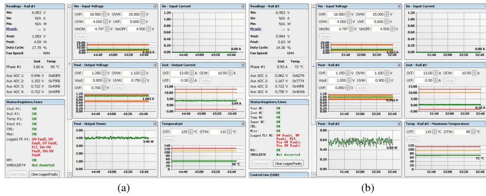
Figure 5: Live parameters monitoring for the power rails: (a) CVDD, (b) CVDD1.
