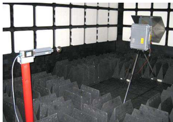
Figure 7: The view of laboratory stand for measurement of HPEM pulse in anechoic chamber.
