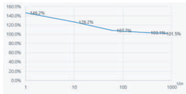
Figure 2: Restoration measurement after 60% elongation at RT.
