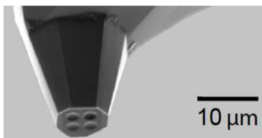
Figure 1: An electronmicroscope image of an AFM tip with four microfabricated curved mirrors.
