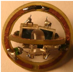
Figure 1: Experimental prototype of the optically coupled meta-atom: one of the broadside-coupled split-ring resonators is loaded with photo-diodes (PD); the other one, orthogonally positioned, is equipped with a light-emitting diode (LED).
