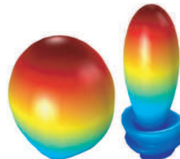
Figure 4: Modelled radiation pattern from patch antenna, and the enhanced directivity achieved via the use of a lens designed via quasi-conformal mapping.
