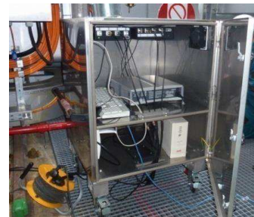
Figure 3: Assembly of the diagnostic system in shielded box.
