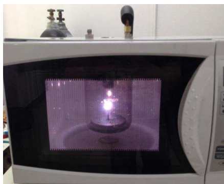
Figure 4: Photograph of plasma generation in ethanol vapor.
