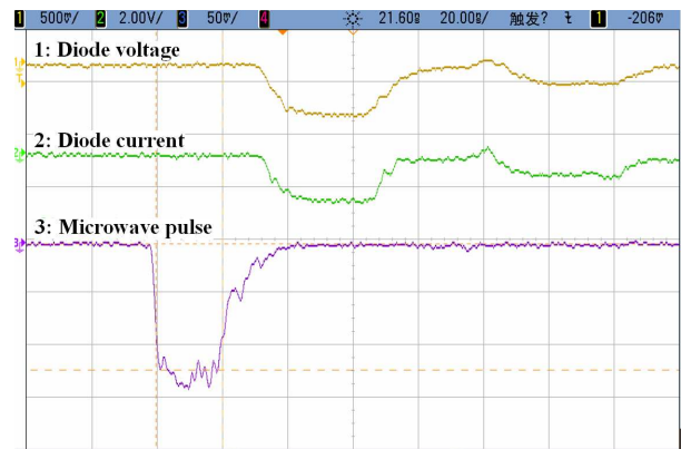
Figure 5: Typical experiment results of CRBWO. Resolution is 20 ns/div on horizontal axis. 1: diode voltage, 505 kV; 2: diode current, 4.26 kA; 3: microwave pulse, 733 MW.
