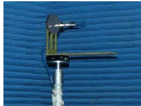
Figure 4: Photograph of the reflectarray prototype into the anechoic chamber.
