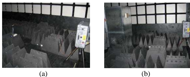
Figure 3: Measuring position for measuring shielding effectiveness with the use of high power generator: (a) standardization measurement, (b) basic measurement.
