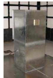
Figure 3: Ventilation panel installed in the real shielding casing.
