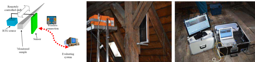
Figure 4: X-ray diagnostic system for monitoring building elements.
