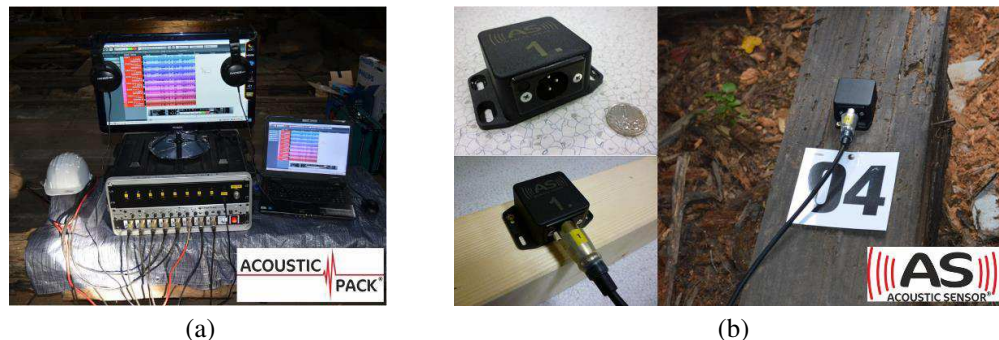
Figure 7: The realized acoustic diagnostic system. (a) Terrain workplace. (b) Detail of the acoustic sensor.
