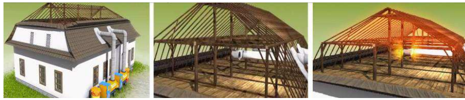
Figure 2: The removal and treatment of wood invaded by wood-destroying insects and fungi.
