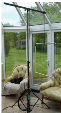
Figure 4: 70 cm square foldable ‘all-coax’ loop-monopole in plastic conduit, suspended to detect reaction forces. (None seen with 700 w RF input.).
