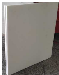
Figure 5: FSS composite structure sample.
