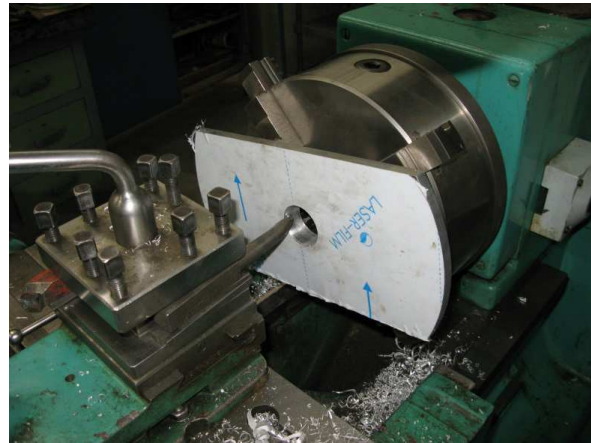
Figure 5: Lathe-turning of the main load-bearing structure of a telescope.
