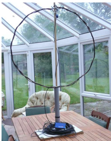
Figure 1: Picture of 90 cm loop-monopole with MiniVNApro (Bluetooth connected) vector network analyser at bottom.
