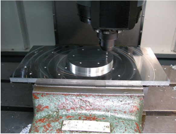
Figure 4: The milling of the surface areas of the main load-bearing part of a telescope.
