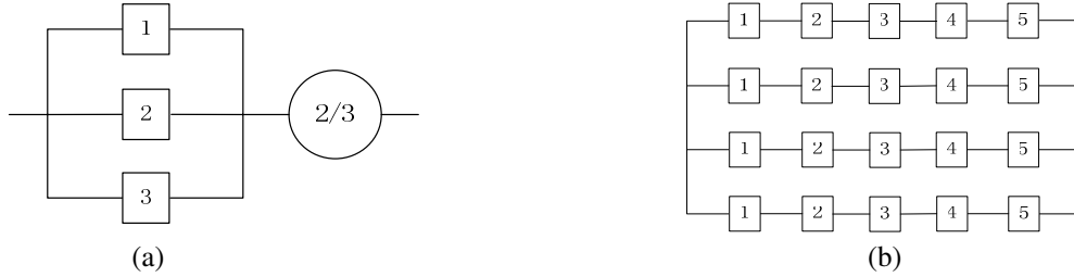
Figure 4: (a) 2/3(G) reliability model. (b) k/n(G) reliability model of the co-phase power supply device.
