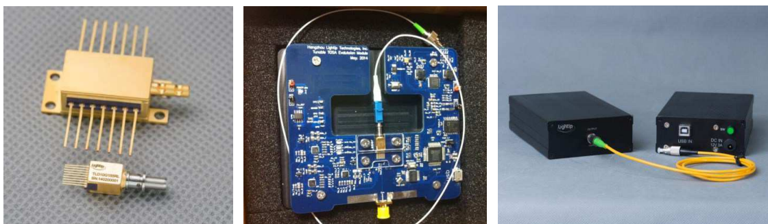
Figure 4: (a) Packaged TOSA module (lower) compared to a conventional butterfly package (upper); (b) An electronic driver circuit board for wavelength control and direct modulation; (c) An enclosed tunable laser module with a USB interface for computer control.
