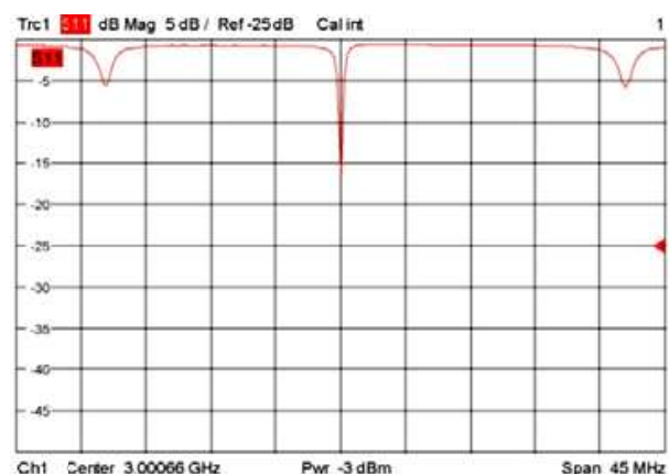
Figure 4: Measured |S_{11}| dB of the LINAC with traditional DW: RL = 16.5 dB.
