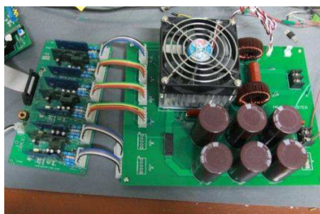
Figure 3: Photo of the PV inverter prototype.
