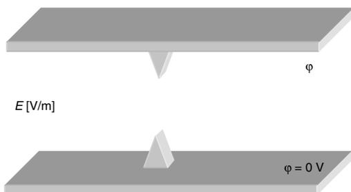
Figure 1: A simple electrical spark gap, 3D.
