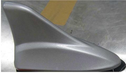
Figure 3: The car FM wire antenna.
