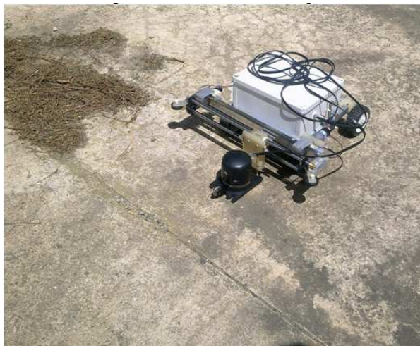
Figure 2: Robotic scanner operating on a concrete pavement. Note the separation line between two concrete pours.
