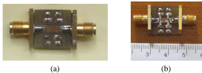
Figure 4: Bandstop small size EBG filter. (a) Without capacitors. (b) With chip capacitors.
