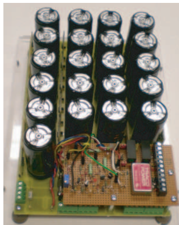
Figure 3: Experimental setup of the energy buffer with electric double layer capacitors (EDLCs).
