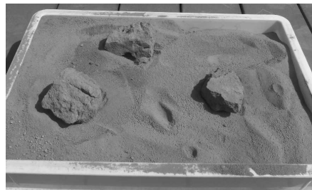
Figure 2: Clods of dried loam soil in the test bed.
