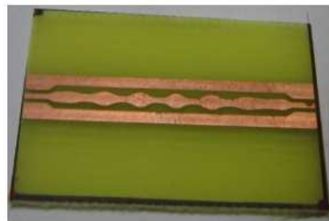
Figure 3: Fabricated structure of CPW on FR-4 substrate.
