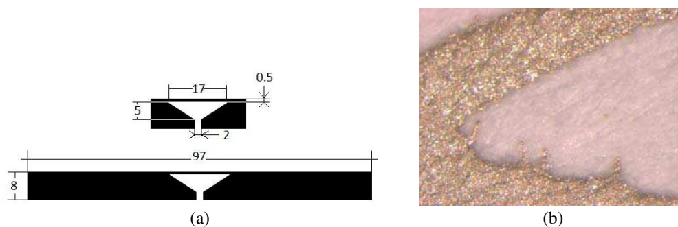
Figure 1: (a) Studied antenna (dimensions in millimetres), (b) sintered antenna on a paper substrate (magnification X57).
