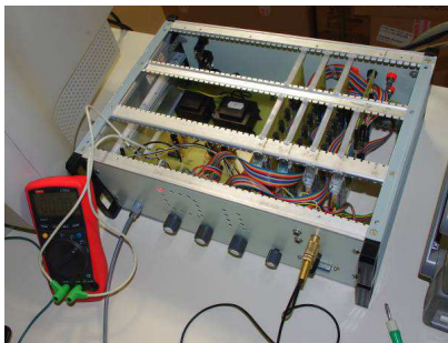
Figure 7: The internal arrangement of the switching unit.
