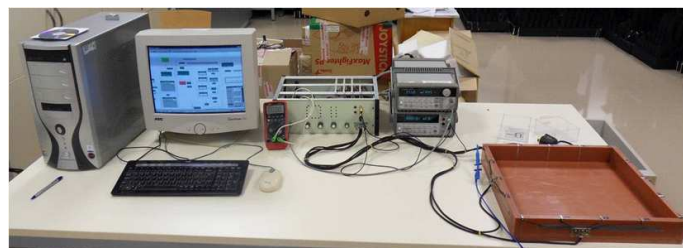
Figure 1: Overall configuration of the measuring system for the EIT method.
