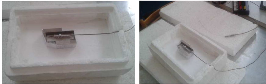
Figure 3: Configuration of the permanent magnets during the experiment.
