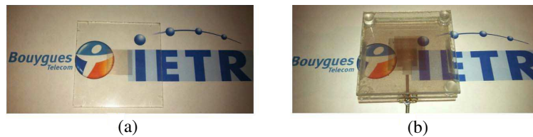
Figure 4: (a) Optical rendering of a varnished glass substrate, and (b) the resulting see-through antenna.
