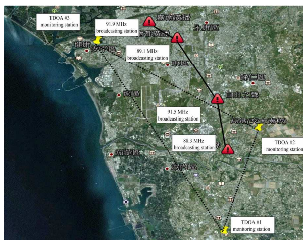
Figure 3: The proposed experiment configuration for investigating the TDOA limitation of location performance in multi-path effect of metropolitan area.
