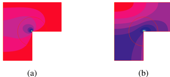
Figure 2: (a) Singular P_S solution and (b) singular electric field ( z -component).
