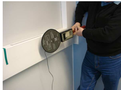
(b) measurement from surface of a transformer
