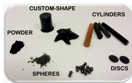
Figure 1: Microwave processing of carbon xerogels permits to design the properties along the final shape of these carbon materials.
