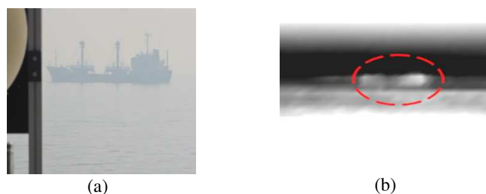
Figure 2: Radiometric measurements at sea: (a) photo and (b) ship image at distance of 1000 m.
