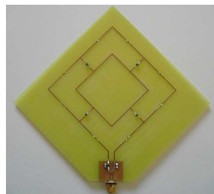
Figure 1: Fabricated prototypes of the loop antennas with left-handed loading.
