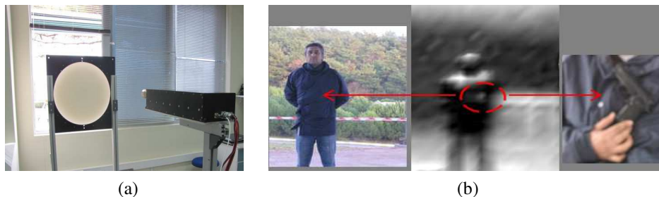
Figure 1: (a) Prototype of passive scanning radiometric system. (b) Photo and radiometric image when scanning weapon concealed under clothing at distance of 10 m, building at distance of 150 m and clouds at the background. The outline of the gun is marked by the dotted line.
