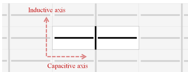
Figure 1: Lerner type geometry adopted for the polariser design.
