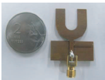
Figure 11: Photograph of the proposed UWB antenna with WLAN band notch.
