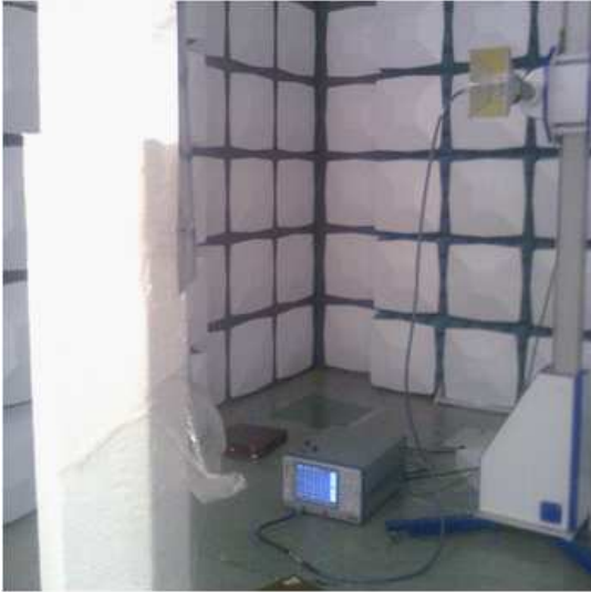
Figure 5: Test setup at electromagnetic laboratory of AUT using ZVK R&S network analyzer.
