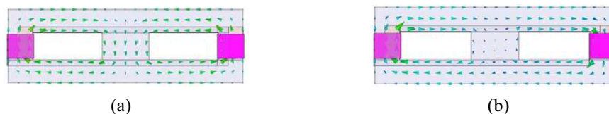
Figure 8: Magnetic flux inside filter magnetic core of FML foils (a) CM excitation (b) DM excitation.
