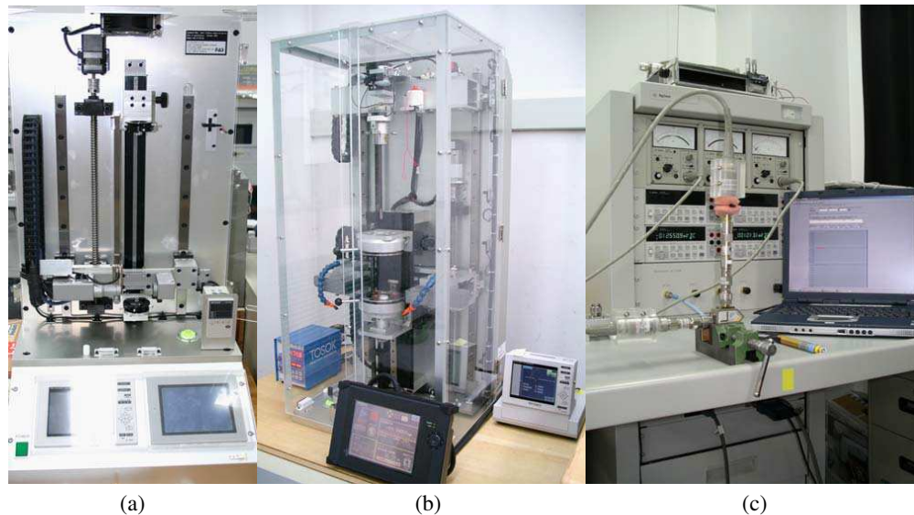
Figure 1: Measurement system for (a) outer diameter of center conductor, (b) inner diameter of outer conductor, and (c) insertion loss at microwave frequency.
