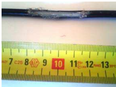
Figure 1: Soft Fault on a coaxial line.
