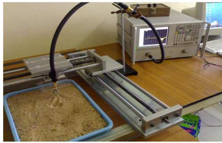
Figure 1: Experimental set up of the Microwave imaging system.
