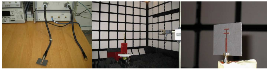
Figure 6: Double T antenna during the measurements in anechoic chamber.
