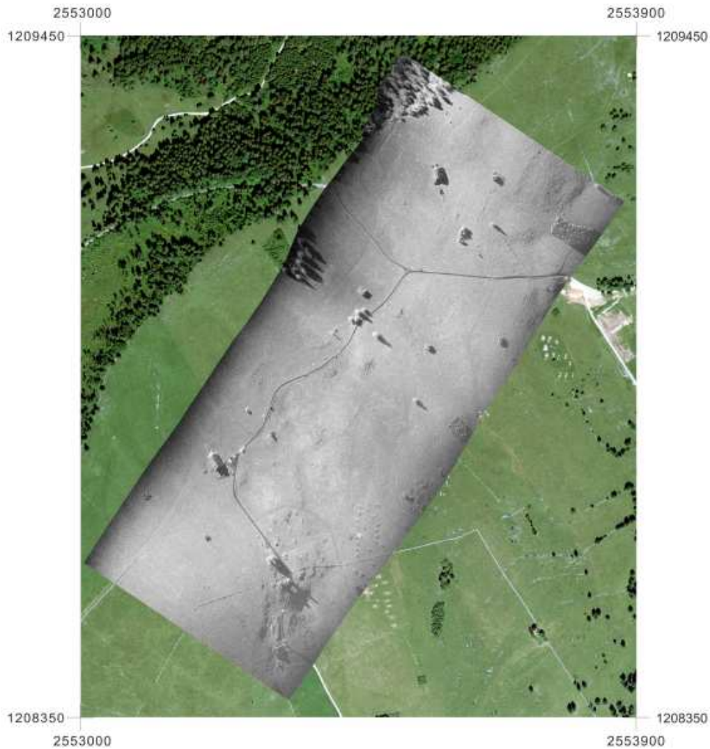
Figure 3: Mosaicked image from the data take 1 in 2011. The SAR image is superimposed over an orthophoto. The coordinate system is LV 95.
