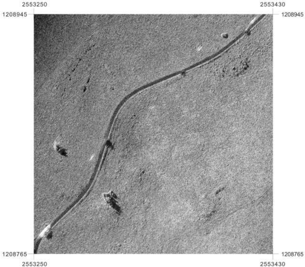
Figure 7: Zoomed view of a geocoded product from the data take 1 in 2011, where the signatures of four moving vehicles are visible. The coordinate system is LV 95.
