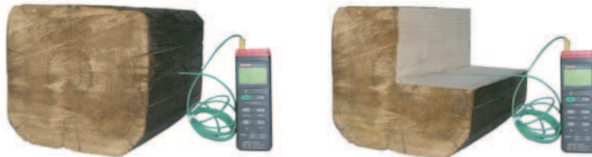
Figure 4: Temperature diagnostics in a section of a wooden structural element.
