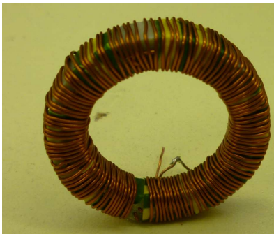
Figure 3: Realized Rogowski coil in form of toroidal coil.
