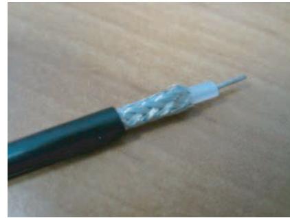
Figure 6: Coaxial cable with shield in the form of copper wire braid.
