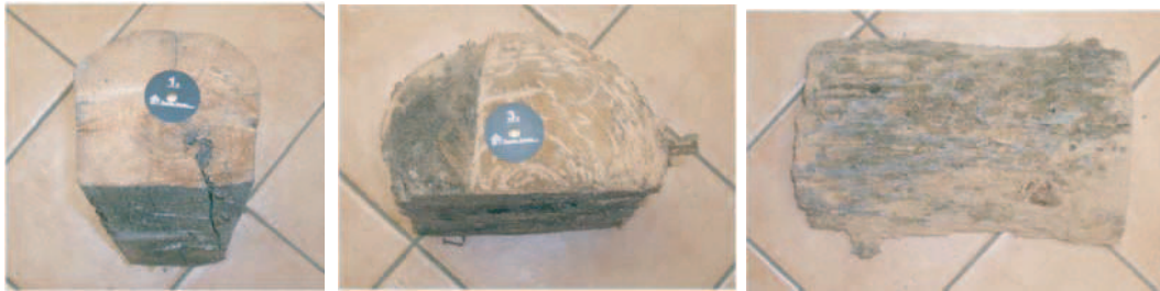
Figure 3: Examples of wood invaded by decay-fungi and wood-destroying insects.
