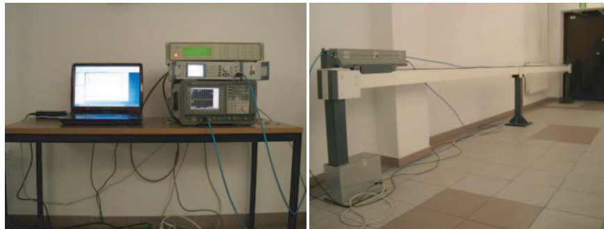
Figure 4: Sample configuration of measuring position to measure shielding efficiency of cable.
