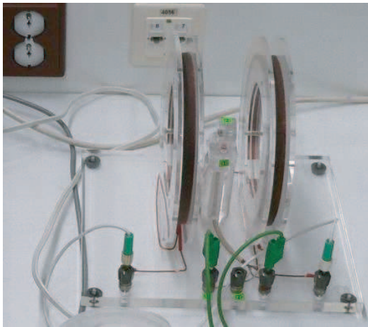
Figure 4: The calibration using Helmholtz coil.
