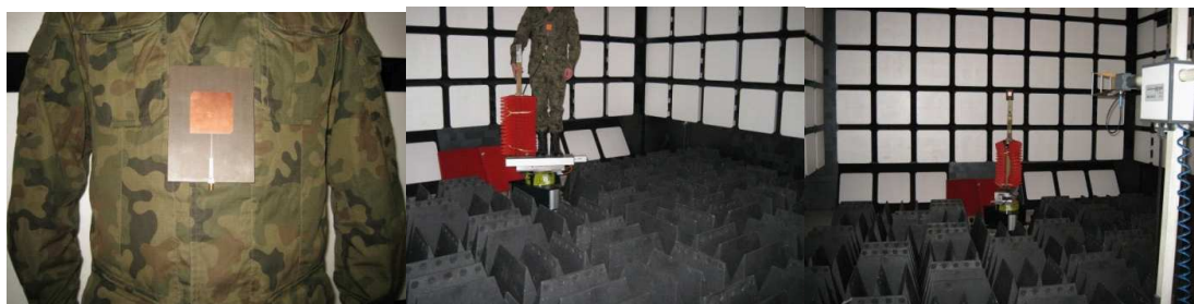
Figure 5: Wearable antenna during the measurements in the anechoic chamber.
