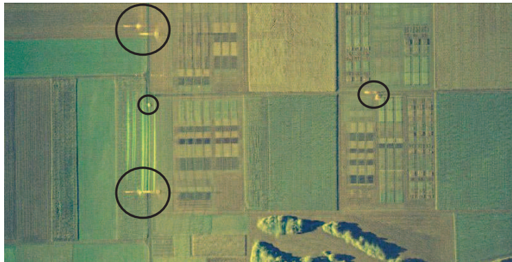
Figure 4: Circular dual-polarization Ka-band composite image of an agricultural area near Oensingen, Switzerland acquired in June 2010. The RR and RL polarizations are respectively represented as red and green channels. Man-made objects appear yellow/red, since they contain more RR scattering due to double-bounce scattering. The electric lines are only reflected once and appear pure green.
