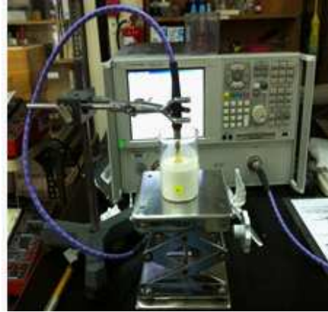
Figure 2: Reflection measurements set-up.
