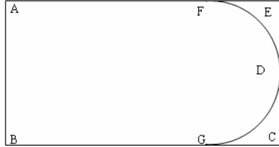
Figure 2: Schematic illustration of the transformation process for the plane wave to convex cylindrical wave.
