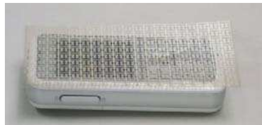
Figure 13: Photograph of slotted FSS film placed on mobile phone for experiment.
