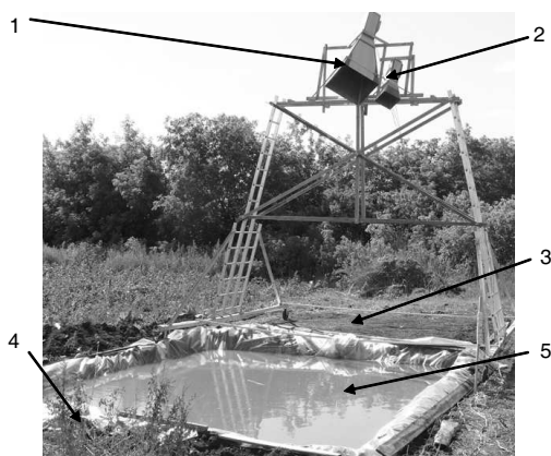
Figure 1: Radiometric installation and test sites view. 1 — 1.4 GHz radiometer; 2 — 6.9 GHz radiometer; 3 — bare soil, 4 — soil covered with grass; 5 — water basin.
