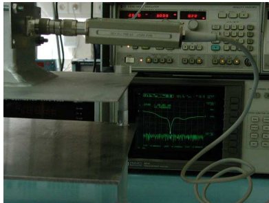
Figure 4: Measurement of S_{11} parameter.
