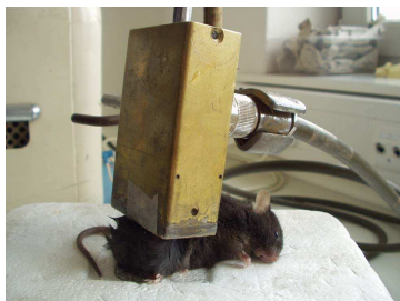
Figure 1: Waveguide applicator for biological experiments.
