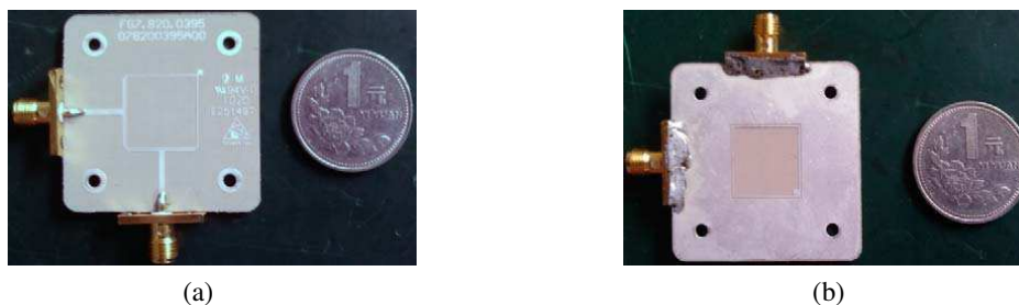
Figure 8: Photographs of the filter. (a) Top view. (b) Bottom view.
