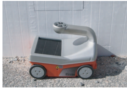
Figure 2: GSSI StructureScan Mini handheld GPR unit used for data collection.
