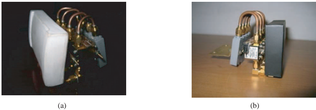
Figure 3: View of model active antenna: (a) Conformal. (b) Planar.
