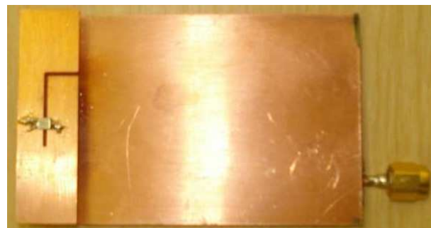
Figure 3: The prototype (loaded) antenna structure.
