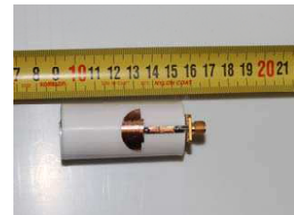
Figure 6: Photograph of the realised half hollow cylindrical UWB antenna.
