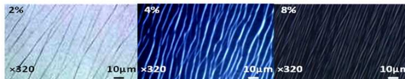
Figure 1: Optical micrographs of PSFLC samples obtained in the isotropic phase ( T = 90^\circ\text{C} ) showing the anisotropic structure of the dispersed network with 2%, 4% and 8% polymer concentrations.
