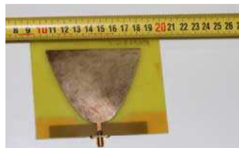
Figure 2: Photograph of the realised planar patch parabolic antenna of y = 0.044x^2 equation.
