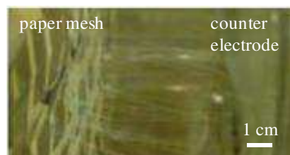
Figure 6: PN fibers formed between the paper mesh and counter electrode.
