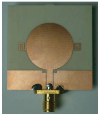
Figure 4: The fabricated band notched UWB antenna.
