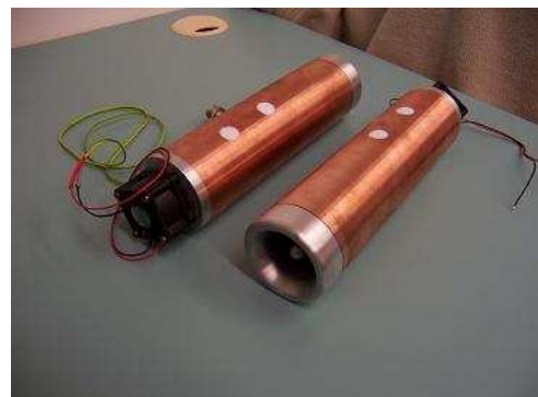
Figure 10: The new gerdien tube designed at the Department of Theoretical and Experimental Electrical Engineering, Brno University of Technology.
