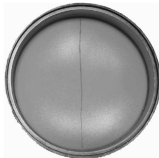
Figure 1: Photograph of a cracked window disk on the vacuum side.
