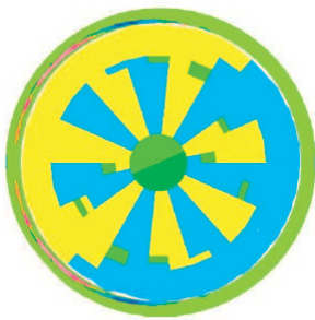
Figure 1: (color online) At time step 50dt , the vertical magnetic flux using GL EMFHS modeling. The GL cloak layer coating materials by AGILD and GL metre Carlo inversion reduce the leakage of the magnetic field.
