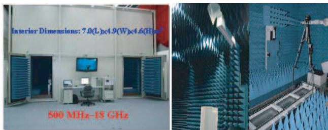
Figure 15: Spherical near-field chamber used for radiation pattern measurement.
