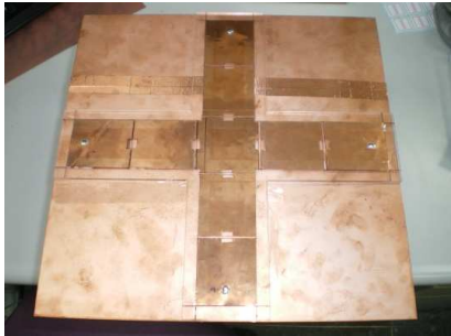
Figure 11: Fabricated cross Yagi patch antenna.
