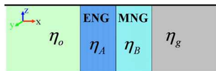
Figure 1: Schematic of an ENG-MNG pair sandwiched between two different semi-infinite regions.
