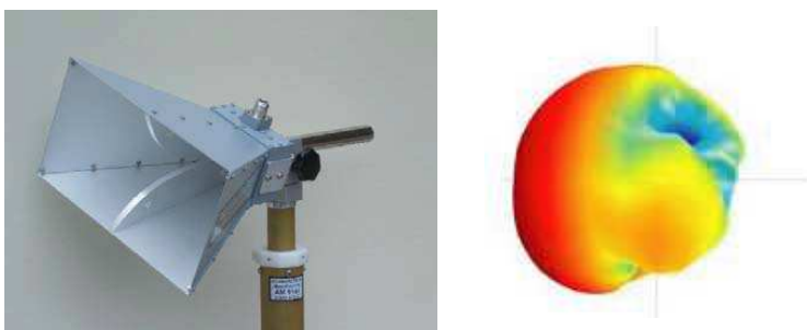
Figure 1: Double ridged horn antenna by 3D antenna measurement.
