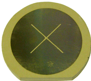
Figure 1: Antenna radiating patch on AD600 substrate.
