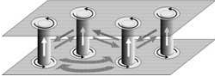
Figure 1: Multiple vias between two horizontal power/ground plates.
